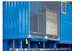
Existing Gottwald Harbour Cranes can be retrofitted to use dynamic brake resistors, which reduces their fuel consumption
