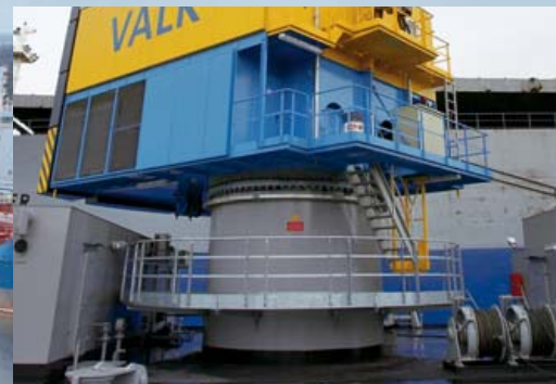
The slew ring of the crane is mounted on a cylindrical pedestal integrated in the barge
