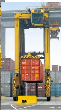
Traffic lights control safe access for straddle carriers
