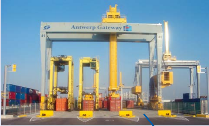
Simultaneous operation of two Gottwald ASCs and fully automated Lift AGVs or manual straddle carriers in the quayside interchange zone
