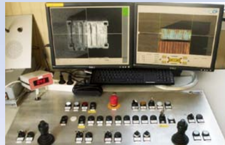
Two general-view cameras and four corner casting cameras guarantee secure, accurate positioning on road trucks on the landside
