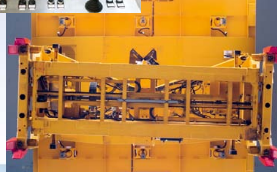
Two general-view cameras and four corner casting cameras guarantee secure, accurate positioning on road trucks on the landside
