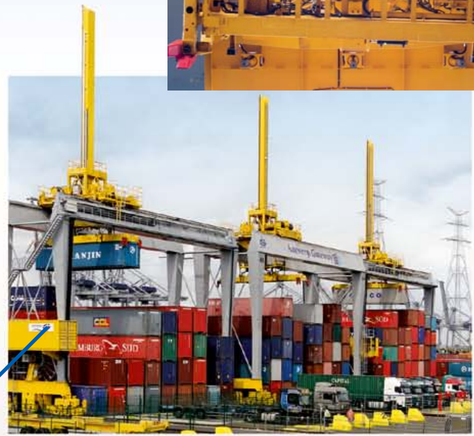
Two general-view cameras and four corner casting cameras guarantee secure, accurate positioning on road trucks on the landside
