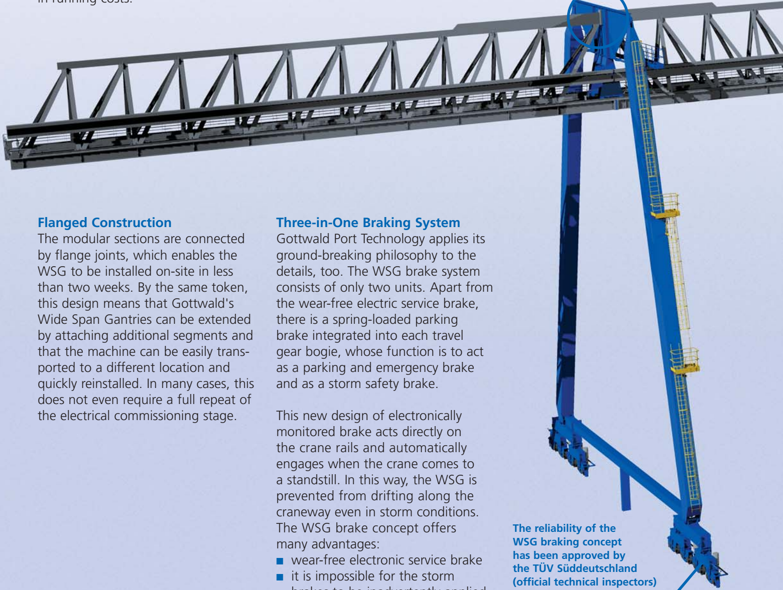
Flanged joints make it possible to install the crane in less than two weeks
