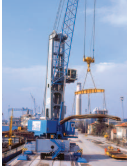
HMK 260 E handling steel wire in the Port of Monfalcone, Italy
