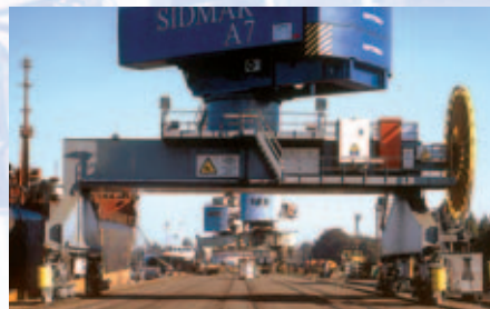
Portal of a Gottwald HSK Portal Harbour Crane using an external power source
