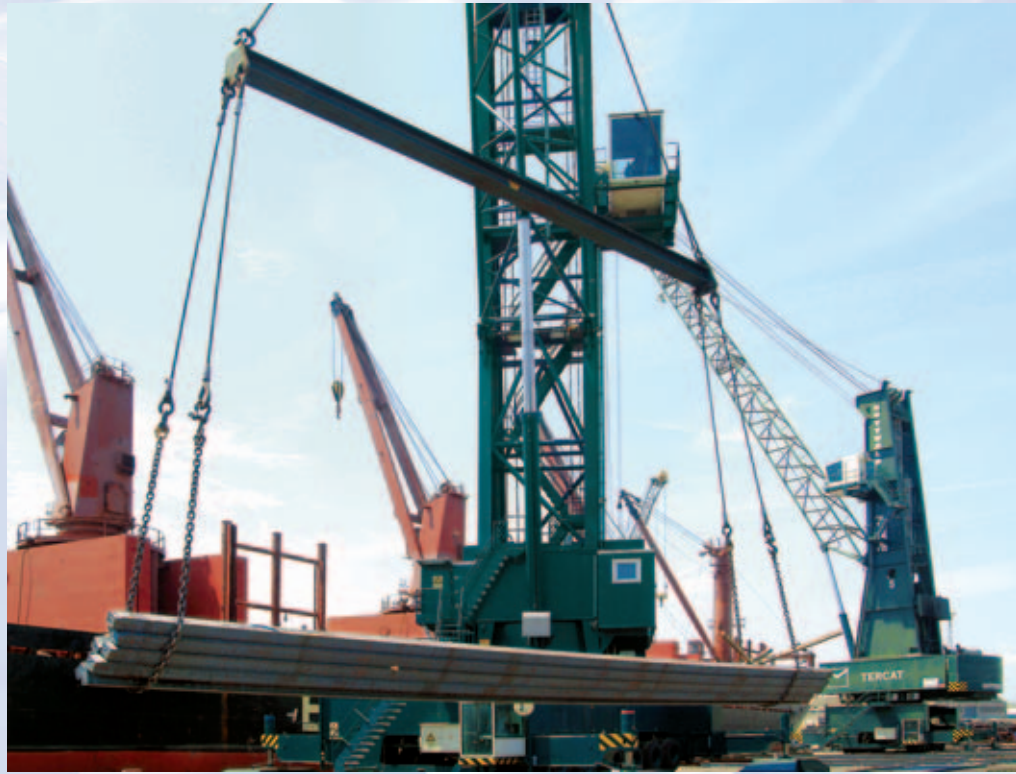
Two HMK 330 EG cranes handling steel billets by means of a lifting beam and chains at Tercat in the Port of Barcelona, Spain
