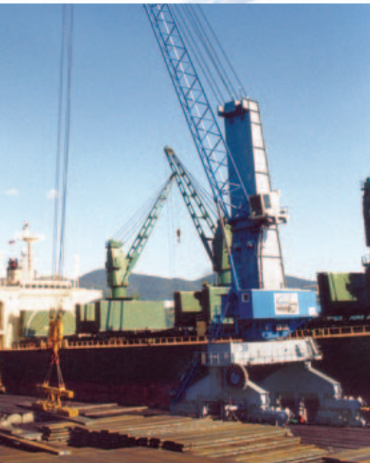
HSK 170 EG with magnetic lifting gear handling sheet steel in the Port of Tuapse, Russia
