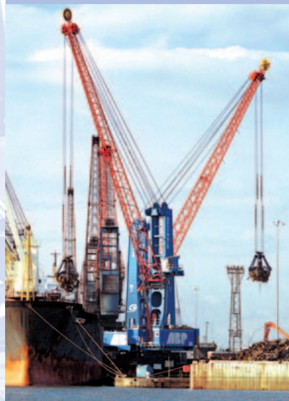
Two HMK 260 EG four-rope grab cranes handling scrap at ABP, Immingham, UK
