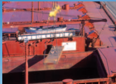
Gottwald HSK 300 E Portal Harbour Crane fitted with a lifting beam handling sheet steel at Sidmar in the Port of Ghent, Belgium
