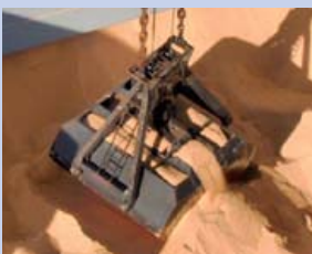
Gottwald Harbour Cranes handle all manner of bulk materials, whether coal, iron ore, gravel, sand, cement, clinker, biomass, animal feed or fertilisers
