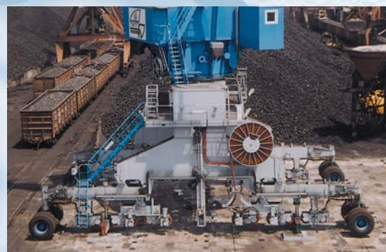
The HSK 170 EG portal fitted with both special travel equipment and 8 stabiliser pads
