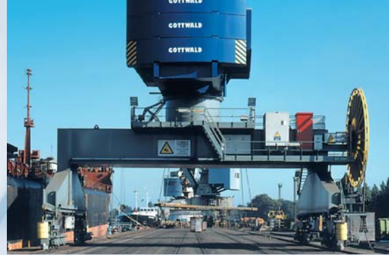
Portals with customised clearance heights and track gauges
