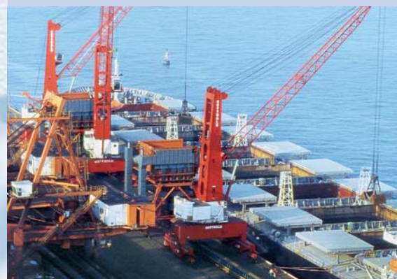
HSK 360 EGL Portal Harbour Cranes with a custom-made portal unloading iron ore at Qinhuangdao, P.R. China
