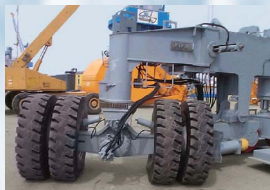
90-degree on-the-spot rotation for excellent manoeuvrability
