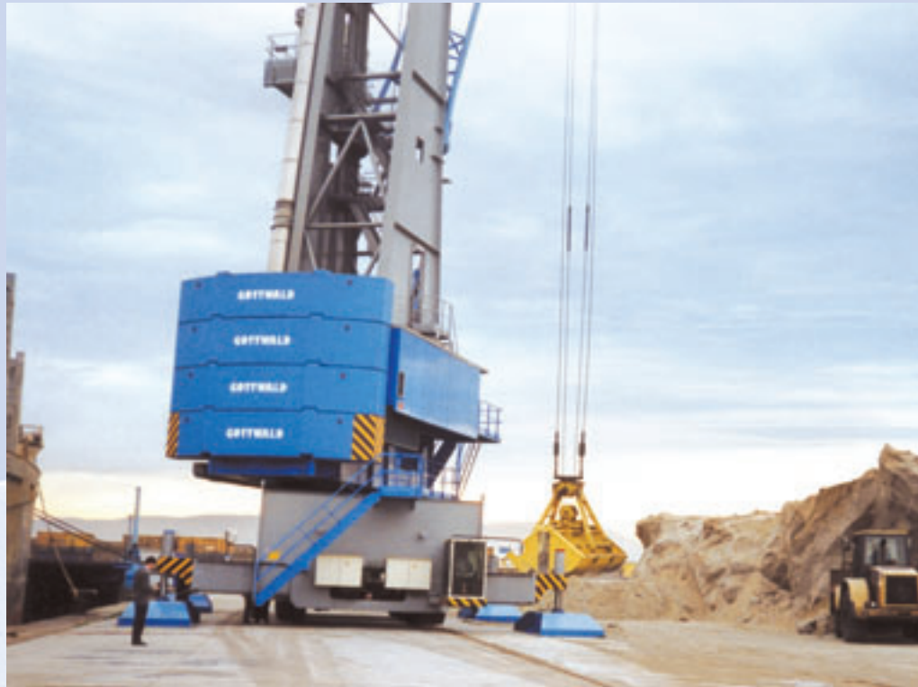
Mobile Harbour Crane with an active dust-protection system handling sand
