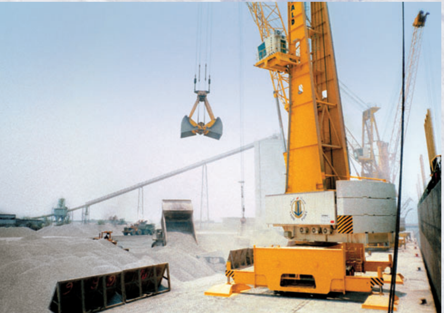
HMK 330 EG handling clinker at Mina Saqr in Ras al Khaimah, United Arab Emirates
