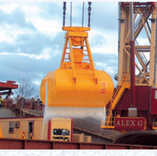
Gottwald Harbour Cranes fitted with 4-rope grab handling fertiliser (top) and soya flour (bottom).
