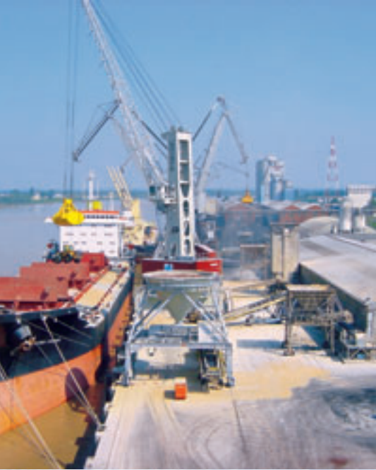
HSK 260 EG discharging soya flour into a rail-mounted hopper in Bordeaux, France
