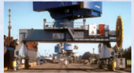
Portal of a Gottwald HSK Portal Harbour Crane using an external power source
