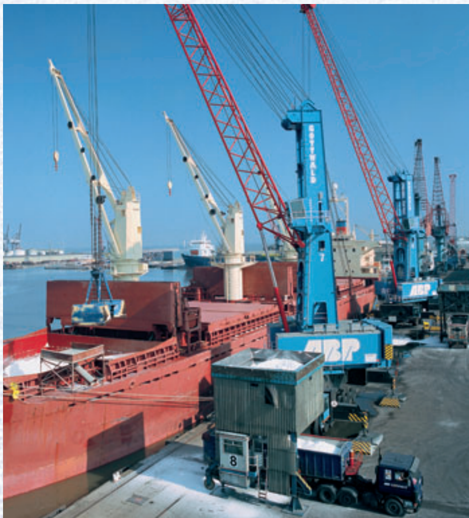
HMK 260 EG discharging fertiliser into a mobile hopper at Humber International Terminal in Immingham, UK
