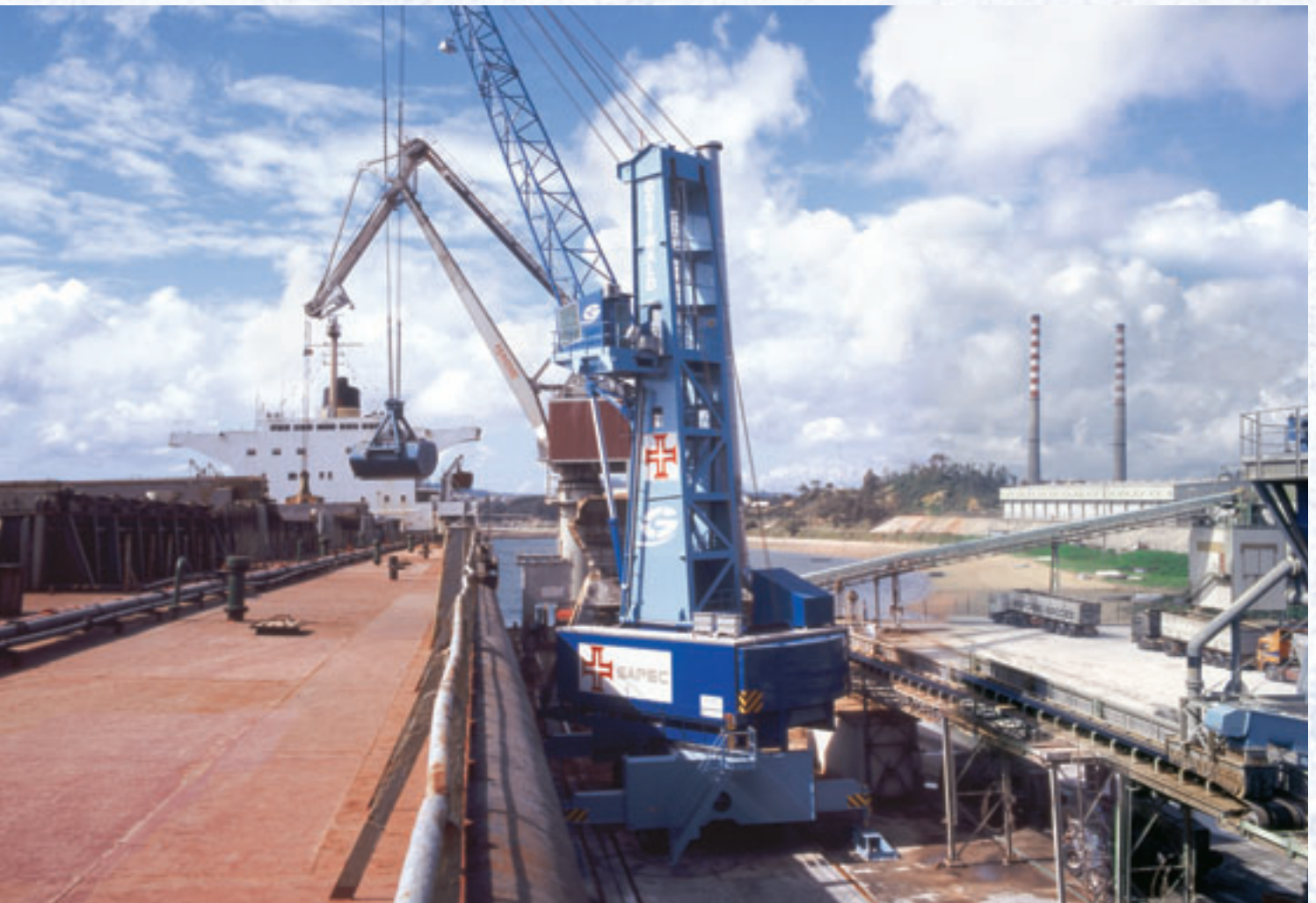
Perfectly integrated into the transport chain of industry close to the terminal: Gottwald HMK 170 EG handling fertiliser with hopper and conveyor belt at SAPEC, Portugal
